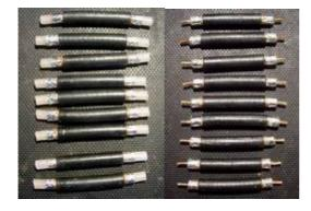
Elements were cut 2% less than the published length to force downwards beam tilting. Elements tinned using 2% silver solder. The dielectric was then cut off and copper ends tinned. Interconnection as shown below. Centre to outside as in the original design in Reference 2.
