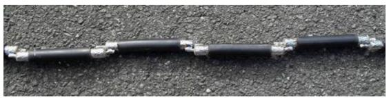
Silver plated wire was wrapped around the connection point for sweat soldering to the copper sleeve balun. A hot plumbers iron was used for a quick solder. This avoids over heating the coax braid and melting the coax dielectric.
