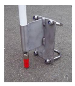
Phil ZL2HF designed a mounting sleeve socket fit for this purpose. This was the first antenna and was later replaced with a longer tail version for ease of connection to the Heliax feeder on site.
