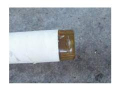
With a high speed cutting disk the resin knob was cut off. The tuning stub could now be adjusted. A sliver plated 3mm diameter wire was used to fine tune the antenna.
