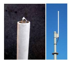
After tuning a new cap is resin filled and placed back on top. A small 2mm hole is required to release the air as it is pushed on. Tape around the hole until the resin has hardened.
